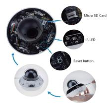
Micro SD card: support insert micro SD card up to 256G.
